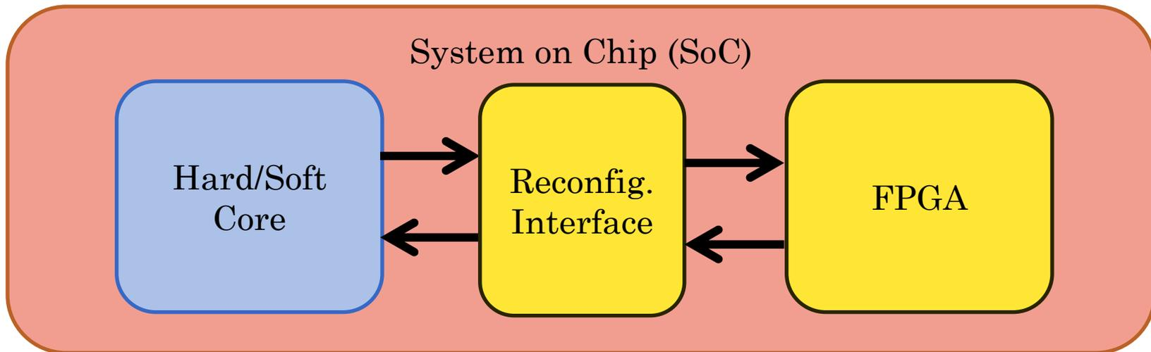
DPR allows the Core to load inside the FPGA the required hardware module only when it is necessary.
