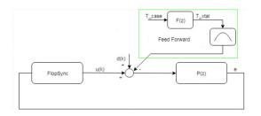
The feedforward temperature compensator is integrated with the FLOPSYNC-2 clock synchronization scheme.
