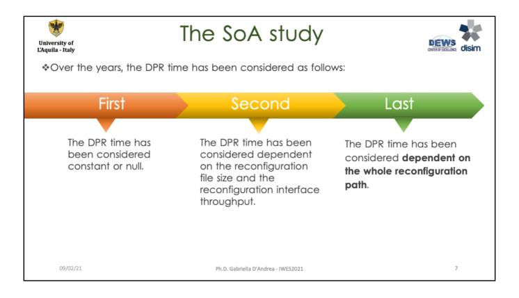
Our DPR time SoA study highlights that does not exist an approach that, considering the whole reconfiguration path (path used to transfer the BS from the external memory to the FPGA reconfiguration memory), allows to calculate in advance the DPR time and it is potentially applicable to all DPR compliant platforms. Hence at this point, we have started working on the reconfiguration path.
