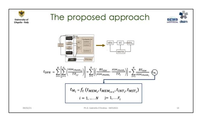
Since at design-time we know both the BS size and the chunk size we can calculate the reconfiguration time considering the features of each component of each elementary path. For example, we can consider the size of the memories, or the interconnections frequencies, or the master command queue depth.
