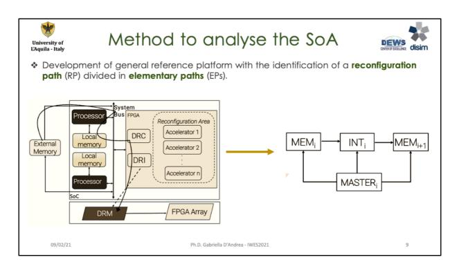
We have developed a general reference platform for DPR identifying the reconfiguration path (indicated in the figure with the black arrow) and dividing it into the elementary path (depicted on the right side of the figure).
