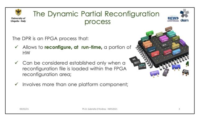
The DPR process requires a certain amount of time to transfer the reconfiguration file, commonly called bitstream (BS), from the external memory to the FPGA reconfiguration area (i.e., FPGA reconfiguration memory).
