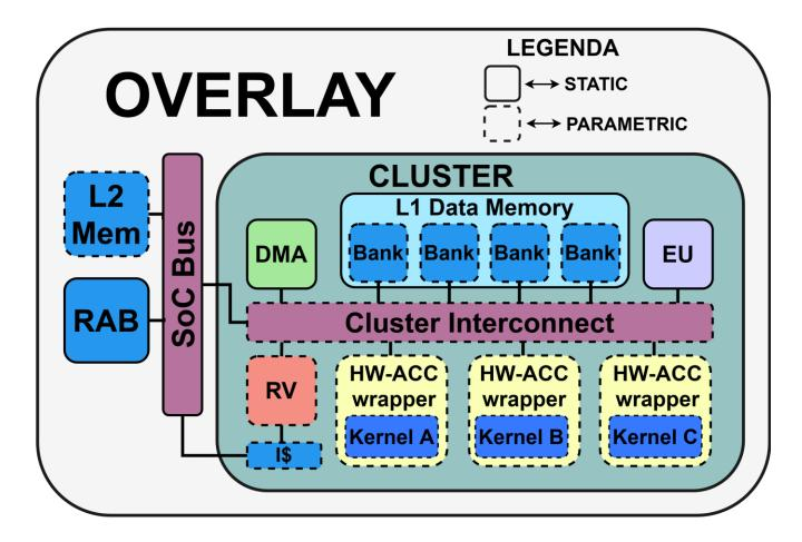
**UNIMORE** An Open-Source Overlay for Reconfigurable, Accelerator-Rich Embedded Systems
