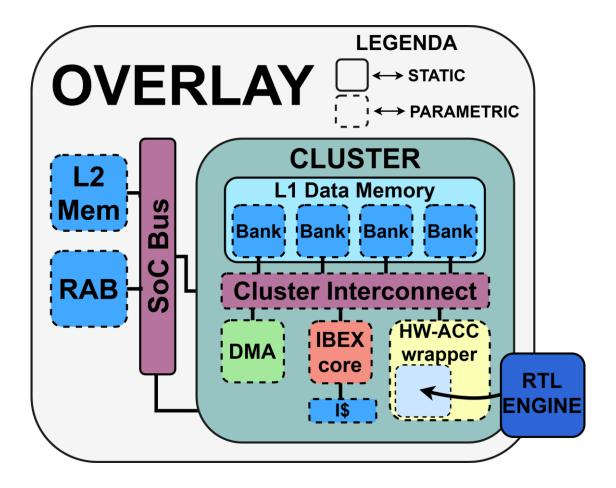
**UNIMORE** An Open-Source Overlay for Reconfigurable, Accelerator-Rich Embedded Systems
