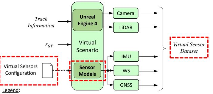
IMU: Inertial Measumerement System; WS: Wheel Sensor; GNSS: Global Navigation Satellite System
